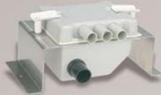
Silencer for wall mounting reduces the high frequency whistle from the suction motor up to 4 dB. Silencer without filter is designed for use when exhaust from the suction is outside of the surgery. Silencer with HEPA filter is designed for use when exhaust from the suction is inside of the surgery.
